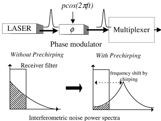
Fig. 7. Principle of reduction of interferometric noise by prechirping.
