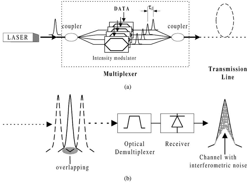
Fig. 1. Interferometric noise in OTDM transmission system. (a) OTDM transmitter. (b) OTDM receiver.
