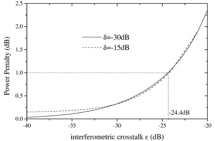
Fig. 3. System performance in the presence of interferometric crosstalk and intersymbol crosstalk.
