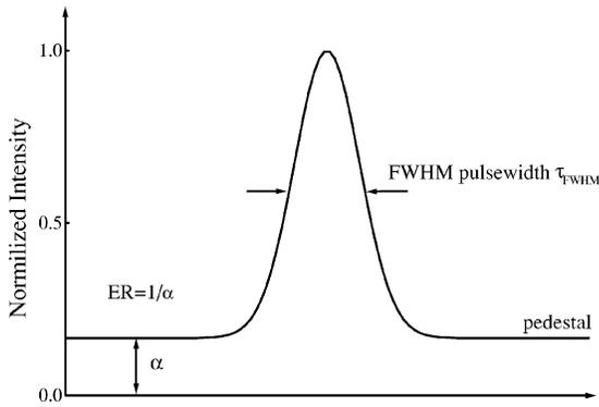
Fig. 4. Parameters used for pulse characterization.
