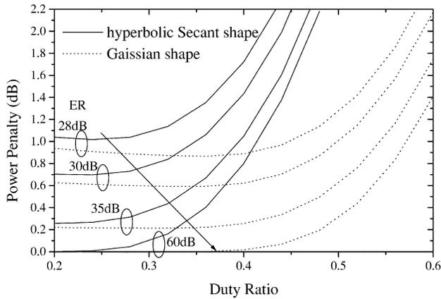
Fig. 5. Power penalty versus the pulses with different pulsewidth and extinction ratio.
